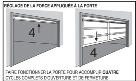
FAIRE FONCTIONNER LA PORTE POUR ACCOMPLIR QUATRE CYCLES COMPLETS D'OUVERTURE ET DE FERMETURE.
