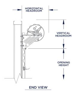
Universal mount 3" deep 12-gauge galvanized steel guides require no pre-installation modifications for wood, steel, concrete or masonry block applications.
